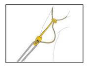
The system enables multiple setup configurations on the branch: wrap-around or choked.
